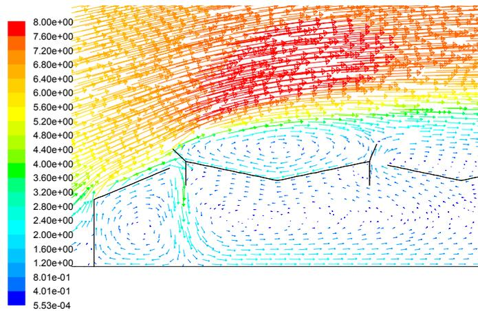
Figure 1(b). Air velocity vector field ( $\text{m s}^{-1}$ ) in the first two windward spans of configuration 2(b).
