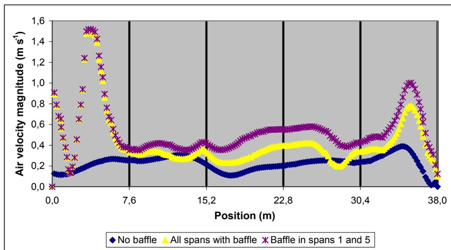
Figure 2. Air velocity values ( $\text{m s}^{-1}$ ) at a height of 1.5 over the greenhouse floor, at different distances from the windward side-wall.
