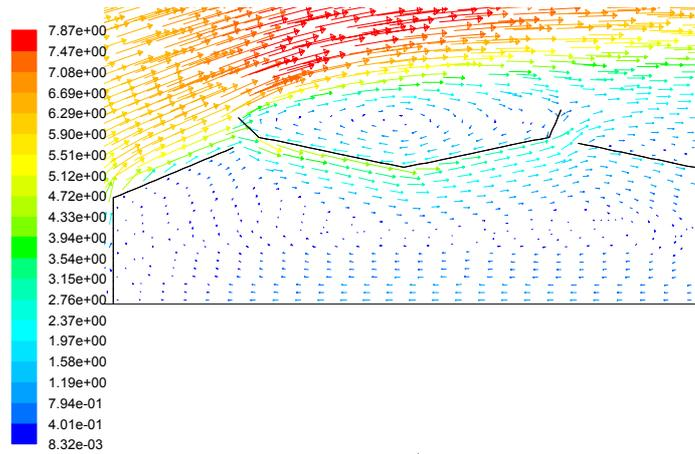
Figure 1(a). Air velocity vector field ( $\text{m s}^{-1}$ ) in the first two windward spans of configuration 2(a).
