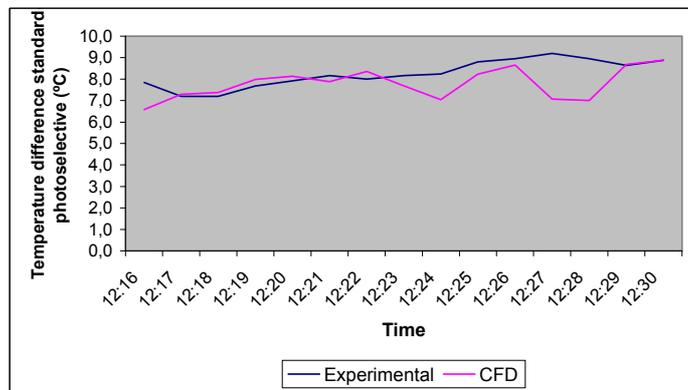
Figure 5. Evolution of the experimental and CFD simulated temperature difference (°C) between both compartments.
