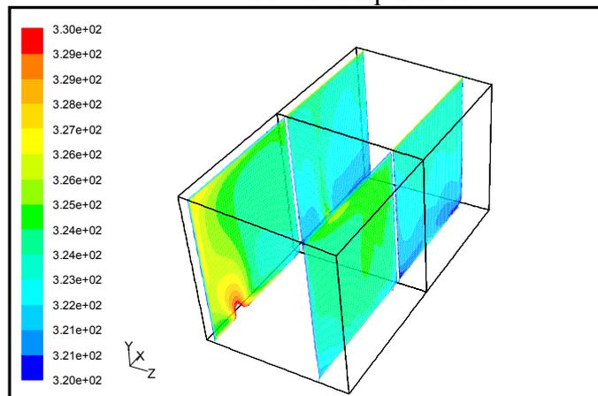
Figure 6. Absolute temperature vertical contours in both compartments.
