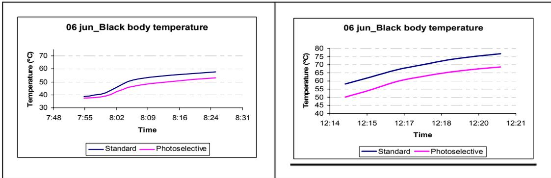
Figure 3(a), (b) and (c). Evolution of the black body temperatures under both materials (standard and photoselective) at different times
