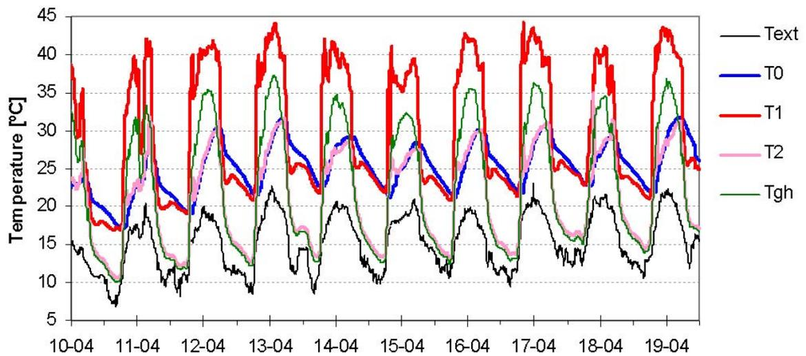
Fig. 2. Temperatures in the system during April 2005.  $T_{\text{ext}}$  = air temperature of the environment,  $T_0$  = average storage temperature,  $T_1$  = air temperature at cooling duct entry (top of tower),  $T_2$  = at cooling duct outlet (bottom of tower),  $T_{\text{gh}}$  = in the greenhouse.
