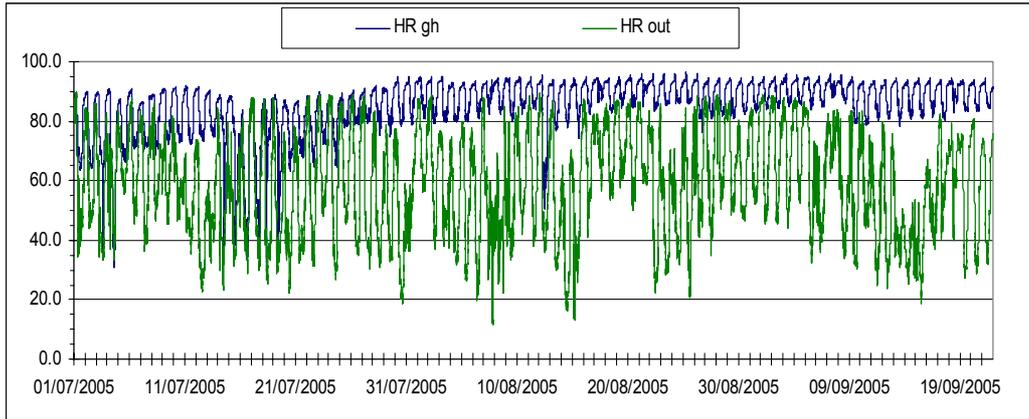
Fig. 5. Relative humidity of the greenhouse (HR gh) compared with the ambient (HR out) July - September 2005.
