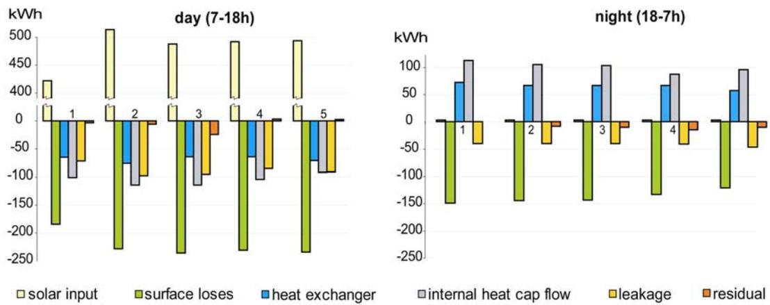
Fig. 4. Energy balance of the greenhouse.
