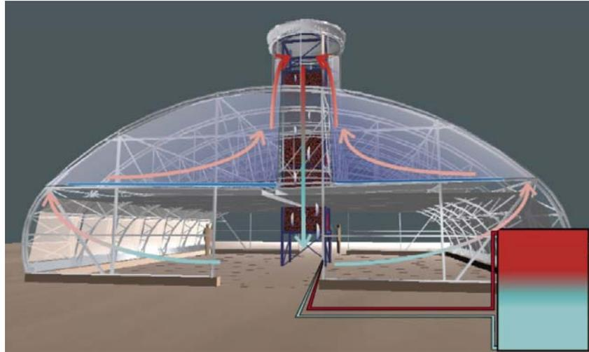
Fig. 1. Air flow scheme of the Watery greenhouse.
