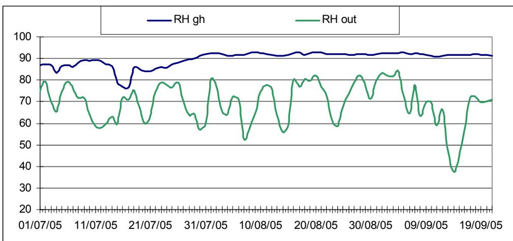
Fig. 7. Mean values of relative humidity in the greenhouse (RH gh) compared with the outside (RH out) during the night through the summer 2005.
