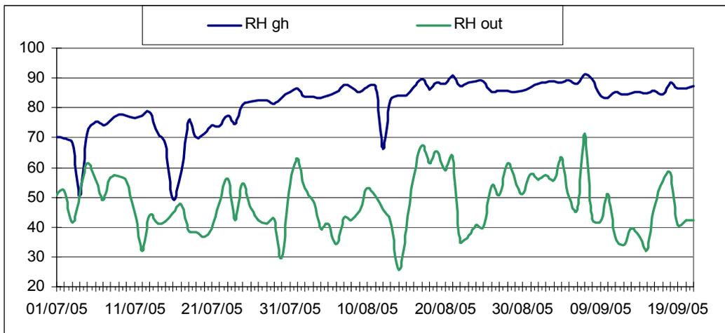
Fig. 6. Mean values of relative humidity in the greenhouse (RH gh) compared with the outside (RH out) during the day through the summer 2005.
