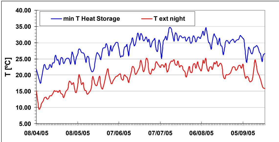
Fig. 3. Minimum temperature of the heat storage compared with outside temperature at night through summer 2005.
